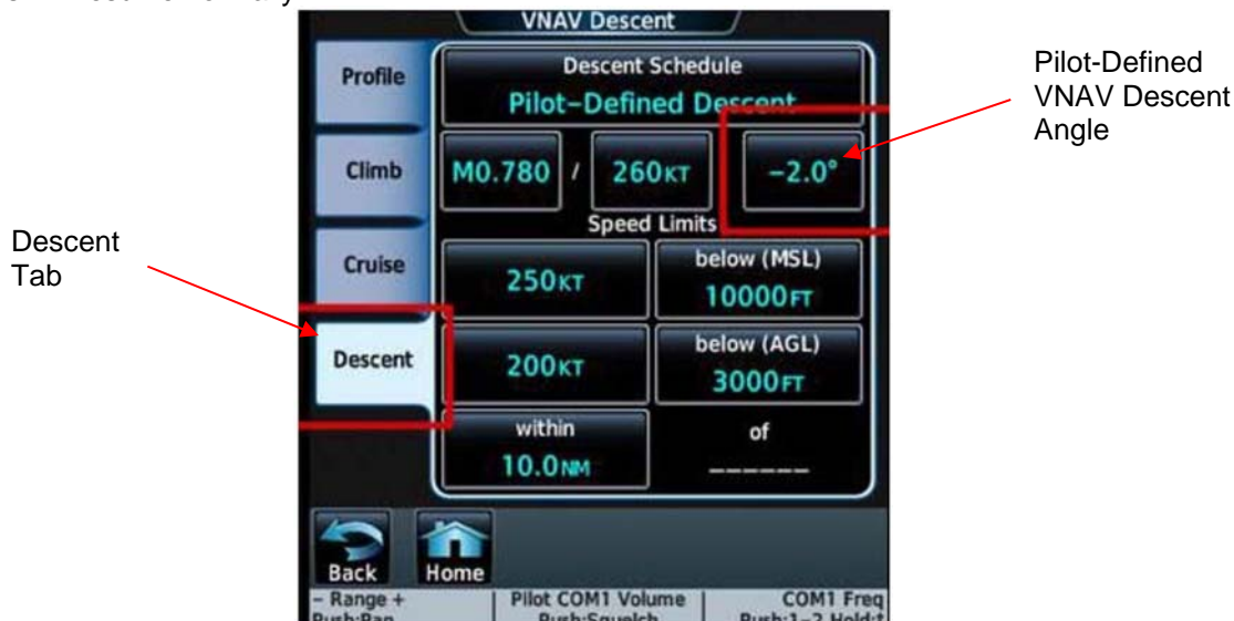
Figure 1 – Descent Tab of the VNAV Profile Page Showing the VNAV Descent Angle
